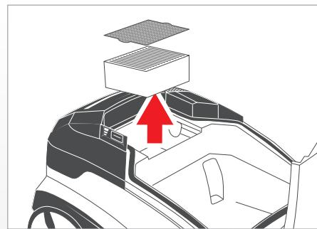
**ⓘ** When cleaning, do not use any brushes or implements which could damage the filter ribs. Before inserting back into the appliance, the filters must be completely dry.
