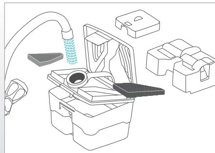
If heavily soiled, you can remove the ejector for cleaning by turning the port gasket.
