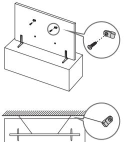
1. Using the appropriate screws, firmly fasten a set of brackets to the wall. Confirm that the screws are firmly attached to the wall.
